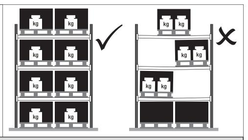
**IMPORTANT!** Pallet Racking must be installed in a combination that is at least 2 bays in length. Single, stand-alone bays and bays with single beam levels are not recommended.
