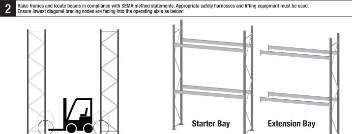
Fit the first beam into the frame by locating the hooked connectors into the perforations on each upright. Ensure the beam is located evenly in both frames and then knock into place with a rubber mallet. Fit beam safety clip as shown below. Repeat the above steps to fit remaining beams. Access equipment will be required for fitting beams at high levels.
