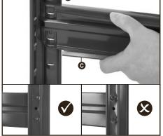
Add remaining Front & Back Beams B 5 to the side frames to create the rest of the levels. Ensuring all beams are at the same height.
